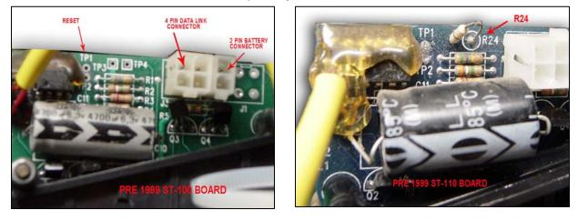
The pre-1999 ST-110 circuit board can be upgraded for use with a Route Wand or Super Wand by clipping resistor R24 from the circuit board and installing a gray cable, 4 wire, upgrade datalink.
